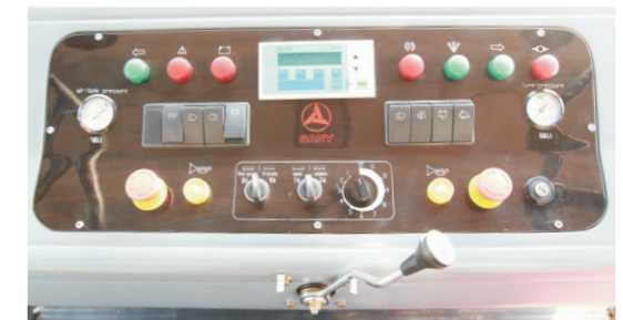
Gear shift switch on operation panel
