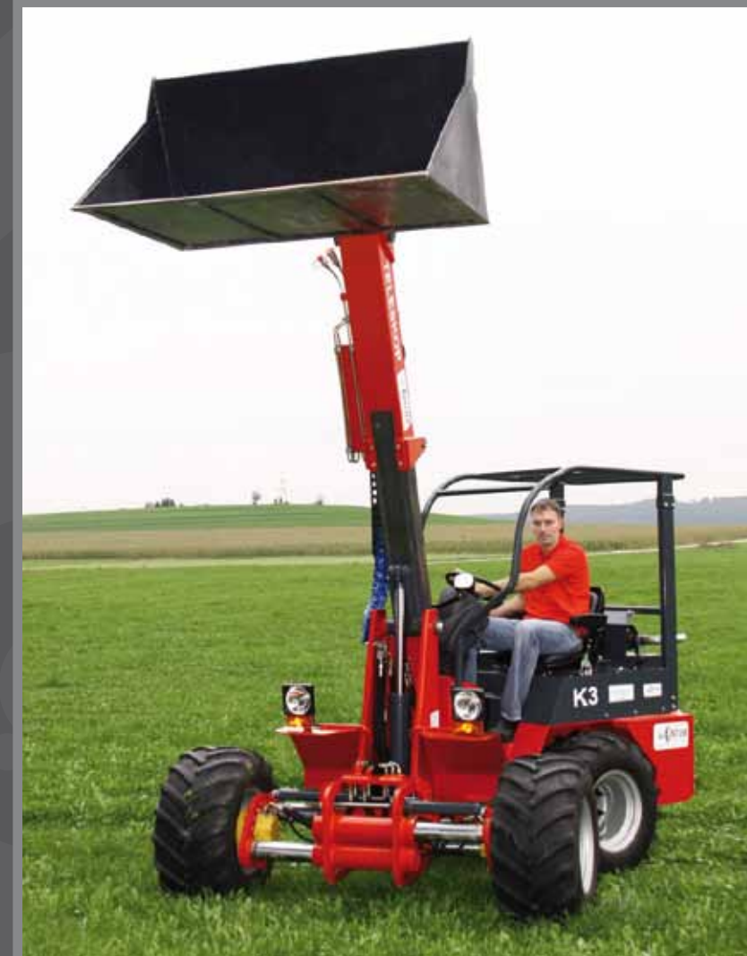
Thanks to the tool holding fixture, which meets the DGS Euro standard, commercially available tools can be used.
