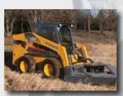
POWER UP ▲ with a 70.7-hp, turbocharged diesel engine with 206 ft.-lbs. of torque, and a rated operating capacity of 2,700 lbs.
