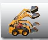
VERTICAL-LIFT ▲ design delivers extended reach and 130-inch lift height, higher than any competitor in its weight class.
