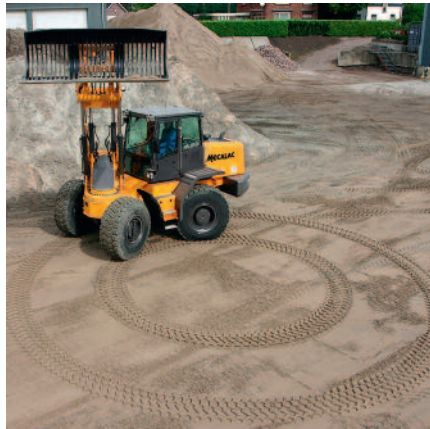
4.90 m turning radius measured over rear end
