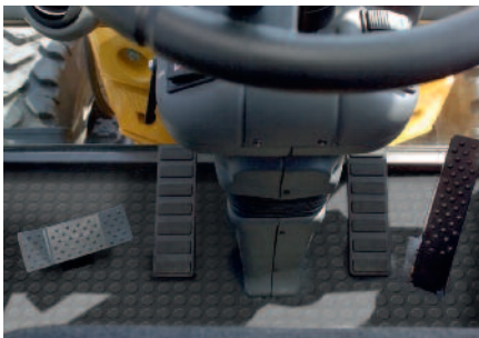
Left foot operated swing pedal avoids tiredness
