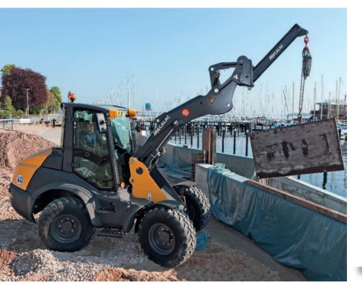
The slender monoboom allows for an optimum view on the attachments. Cylinders, hoses and electrics are protected inside the boom. This extends the life of components and reduces maintenance and repair costs.
