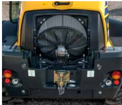
Tiltable radiator fan for convenient cleaning access
