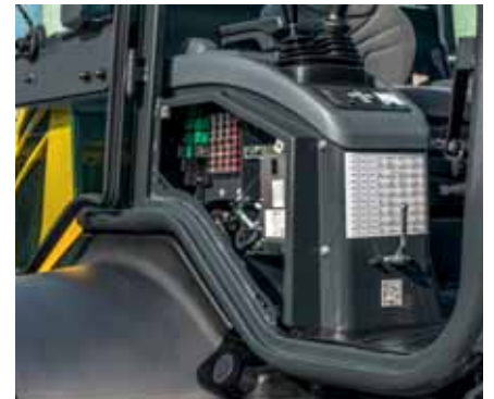
Side cover for quick maintenance access
