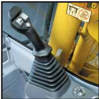
Joysticks with proportional control button for attachments
