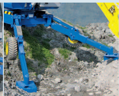
Telefuss Continuously extendable telescopic legs of 850 mm (2.8 ft.)
