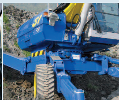
Undercarriage Robust undercarriage with additional fuel reservoir of approx. 58.7 us gal. (100 litres)
