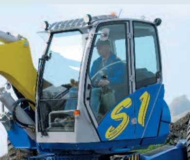
Modern cabin Comfortable and wide cabin, functional cockpit, excellent all-over view (ROPS-FOPS proofed)
