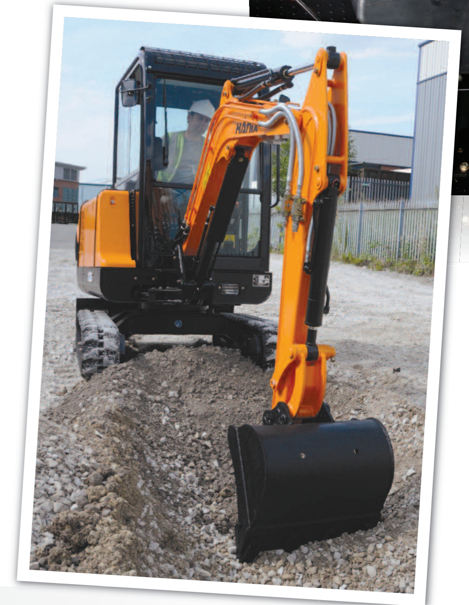
Long 'X' track frame with generous ground clearance provides strength and versatility in all conditions.
