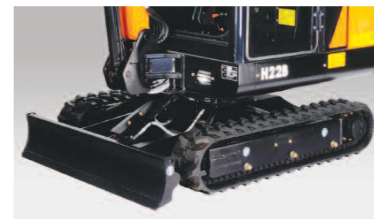
Long 'X' track frame with generous ground clearance provides strength and versatility in all conditions.
