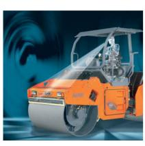
075K ASC - Articulated tandem roller with vibratory and oscillating drum
