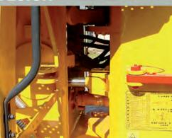
Widely spaced upper and lower hinge pins pivot on double-tapered roller bearings. The hinge plates are designed to allow stresses to smoothly dissipate into the frame. Special applications often require different buckets and tools. Dressta offers high lift arrangements, log grapples, fork-lift attachments and tool carrier arrangements to meet your needs. ecificatio
