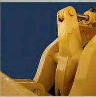
Z-Bar linkage transfers maximum force to the bucket to pry out har material. All loader linkage pins a to keep out abrasive dust and gri
