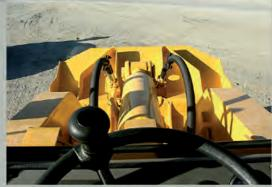
Independent box section booms provide more strength with less weight on the front end of the machine. This improves machine stability, provides less tire loading and lowers tire heat generation in load and carry applications. High strength castings at each end of the boom arms distribute stresses and ensure thousands of hours of trouble free life.
