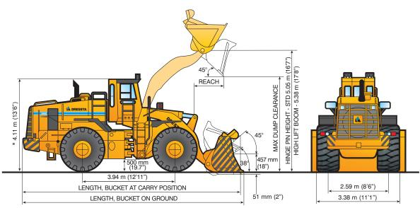
\*Add 240 mm (9.5") to overall height if roof mounted lights are used
