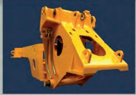
The frame weldments are made from high strength steel and incorporate castings at critical locations to absorb heavy weights shock loads and racking forces.
