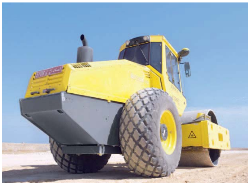
Customised for individual site work: totally enclosed engine compartment.
