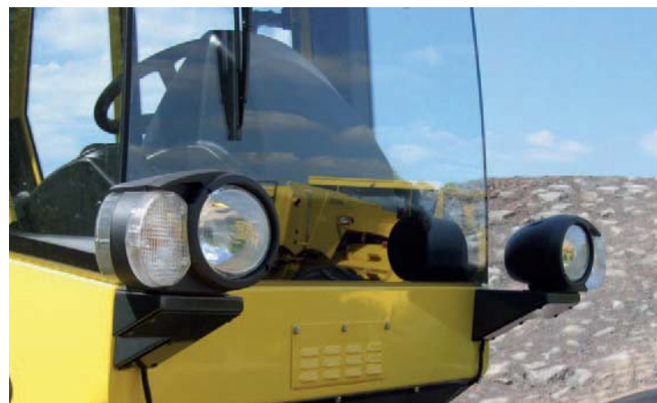
Federal motor safety standard lighting for safe use on roads.
