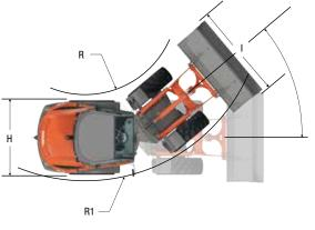
5250 mm 2475 mm 1765 mm С 3930 mm C1 3130 mm C2 2475 mm D 85 mm Ε 670 mm 440 mm G 2000 mm 1785 mm 1850 mm R 1840 mm R2 3690 mm 40°
