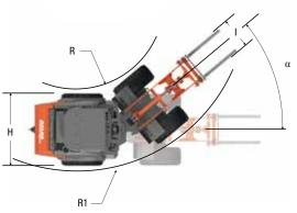
4855 mm B1 1696 mm B2 2380 mm B3 2447 mm 3325 mm С 2725 mm C1 C2 1180 mm D 75 mm Ε 245 mm E1 1010 mm E2 565 mm 400 mm G 1715 mm 1500 mm 1030 mm 1605 mm R1 3150 mm
